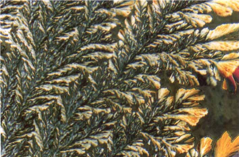
Figure 6. Arborescent structures observed for TSUHPC/DMAC solutions at about 25^{\circ}\text{C} between crossed polars ( \times 680 ).
