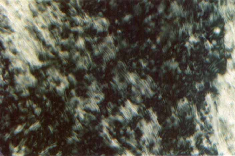
Figure 5. Photomicrograph of fingerprint pattern for the TSUHPC/acetone liquid crystal phase between crossed polars ( T = 25^{\circ}\text{C} ) ( \times 680 ).
